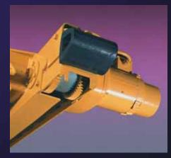
Two driven wheels are used to propel the trolley. The trolley traverse is driven by a TENV motor with a standard AC disk brake. This drives a geared flange, fixed axle wheel with a secondary pinion line shaft connected to a drive pinion in the other end truck.
